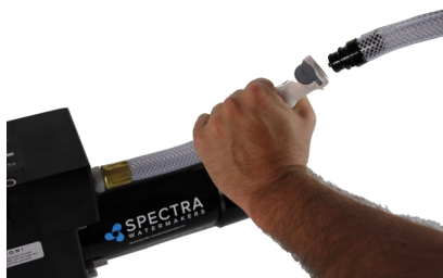
Connecting brine discharge service hose
