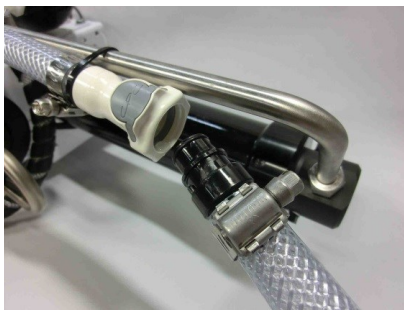
Connecting brine discharge service hose
