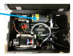
Aquifer Power Pack models are shipped with the battery disconnected. Connect the battery using the large red connectors.
