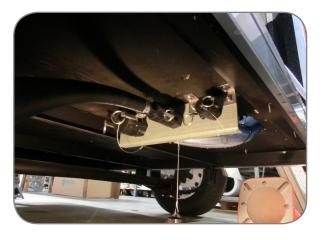
Vents were added to the sides of the trailer, and under the door we added quick disconnect fittings so the unit can move to a safe location during threatening weather.
