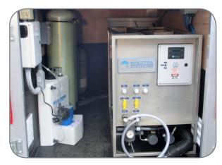
We started with a standard 5 ft. x 8 ft enclosed trailer and added additional components. The interior was coated with a heavy duty spray-on urethane (Rhino lining) to waterproof the floor and walls as well as create a drain tray under the watermaker.
