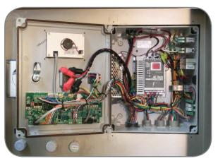
The customer had very specific requirements as to how the control system was to operate so the watermaker was designed with a unique control panel. All electrical controls are well marked for reference. In the left picture is the run timer so the watermaker is only running during the parts of the day where the solar panels are producing power. The various control functions are managed by the watermaker control box with MPC automatic controls and relays.
